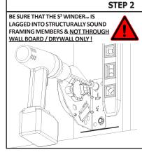
**BEFORE INSTALLING** APPROPRIATE LENGTH 5/16"ø LAG SCREWS SUPPLIED WITH YOUR **GARAGE DOOR, IT IS IMPORTANT TO DRILL** 3/16"ø PILOT HOLES WHERE THE LAG SCREWS ARE TO BE ATTACHED. POSITION THE BOTTOM OF S<sup>3</sup> Winder™ ON THE **LEVEL LINE FROM STEP #1** AND SECURELY FASTEN IT TO A WOOD STUD OR A STRUCTURALLY SOUND MEMBER.
